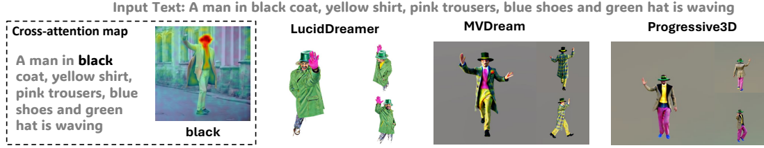
(a) Visualization of cross-attention map. For longer text prompts, 2D Stable Diffusion (SD) [26] fails to accurately associate the word “black” with the correct spatial location in the generated image. This limitation poses a challenge for methods [15, 27] lifting 2D to 3D using SD effectively.
